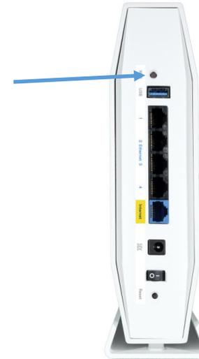
Monitor the MESH LED of both Parent and Child Node. At this time, it should be blinking blue rapidly.
